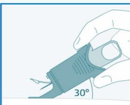
Place your index finger on the top release button and your thumb on the bottom release button. Position AutoSoft™ 30 with its legs level (flat) on the skin to ensure an insertion angle of 30°.
