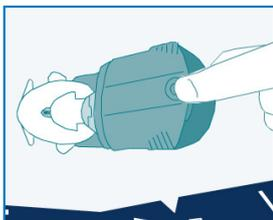
Gently squeeze on the top and underside of the housing to insert the set.
