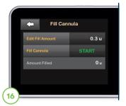
Fill cannula 0.3 units (6 mm cannulas) or 0.5 units (9 mm cannulas). Put the lid back on the insertion device before disposing.
