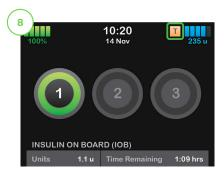
The Screen Lock screen will appear with the orange T icon indicating a Temp Rate is active.
