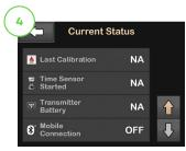
Tap the **Down Arrow** to display the Last Calibration, Time Sensor Started, Transmitter Battery status, and Mobile Connection status.
