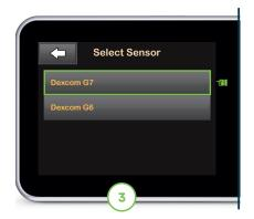
If this is the first time using a Dexcom G7 sensor, tap **Select Sensor** and then tap **Dexcom G7**. Otherwise, skip to Step 4.
