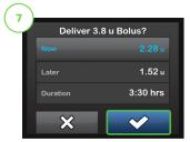
The delivery screen will confirm how much insulin will be delivered up front, how much will be delivered over time, and the delivery duration.
