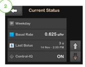
Your t:slim X2 insulin pump will display the name of the user's active profile, the current basal rate, the time and amount of the last bolus, and whether or not they are using Control-IQ technology. If the user has an active Extended Bolus, this screen will show how much insulin has been delivered out of the total amount requested.
