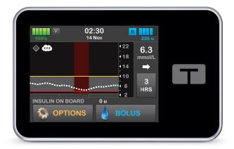
The t:slim X2 insulin pump with Control-IQ technology uses continuous glucose monitoring (CGM)\* values to predict glucose levels 30 minutes ahead and automatically adjust insulin every 5 minutes.
