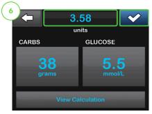
Tap v to continue. Tap the calculated units value to manually adjust recommended dose.
