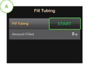
Hold the pump vertically to ensure any air in the cartridge will be dispelled first. Tap START. The pump will beep and vibrate regularly while the tubing is filled.
