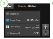
Your t:slim X2 insulin pump will display the name of the user's active profile, the current basal rate, the time and amount of the last bolus, and whether or not they are using Control-IQ technology. If the user has an active Extended Bolus, this screen will show how much insulin has been delivered out of the total amount requested.
