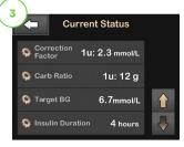
Tap the **Down Arrow** to display the current Correction Factor, Carb Ratio, Target BG, and Insulin Duration.
