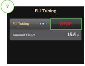
Tap STOP after three drops of insulin are seen at the end of the infusion set tubing, or after a minimum of 10 u have been filled. Verify that drops are seen and tap DONE.
