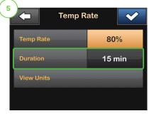
Tap Duration. Using the onscreen keypad enter desired length of time for Temp Rate.
