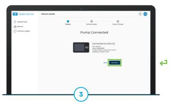
A Pump Connected screen will appear if the connection is successful. Confirm the pump serial number is accurate before clicking **Continue**.
